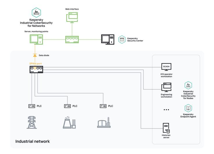
Example Server connection via data diode
