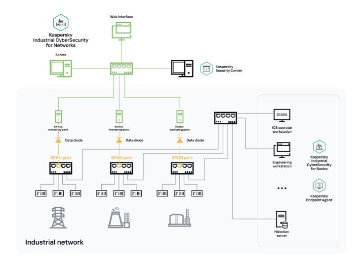
Example connection of sensors via data diodes
